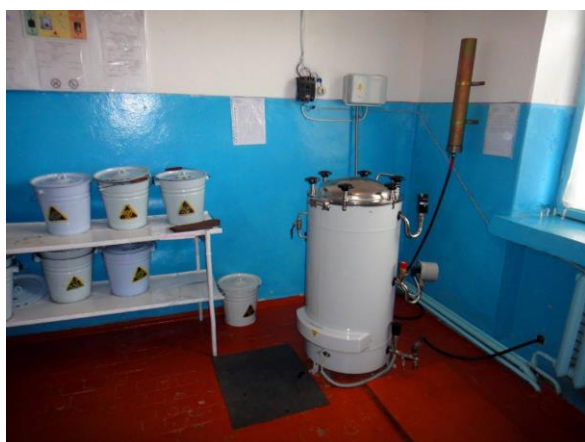
Photo 3: Two buckets will fit directly into the autoclave for sterilisation, thereby minimising the handling of infectious waste.
